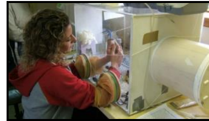
Pore water filtration, separation and conservation treatment in inert atmosphere
