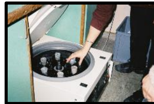
Sediment slices centrifugation in inert atmosphere
