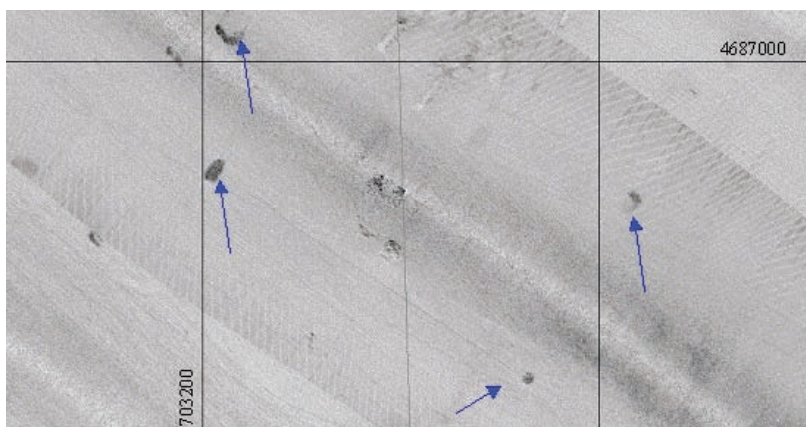
Figure 1.13 – Detail of a morphological relief of a sector situated in the central Tyrrhenian Sea offshore Anzio (central Latium), dredged through a trailer dredge. Backscatter areas ascribable to sand material losses are caused by the dredge's motion (ICRAM, 2005b).
