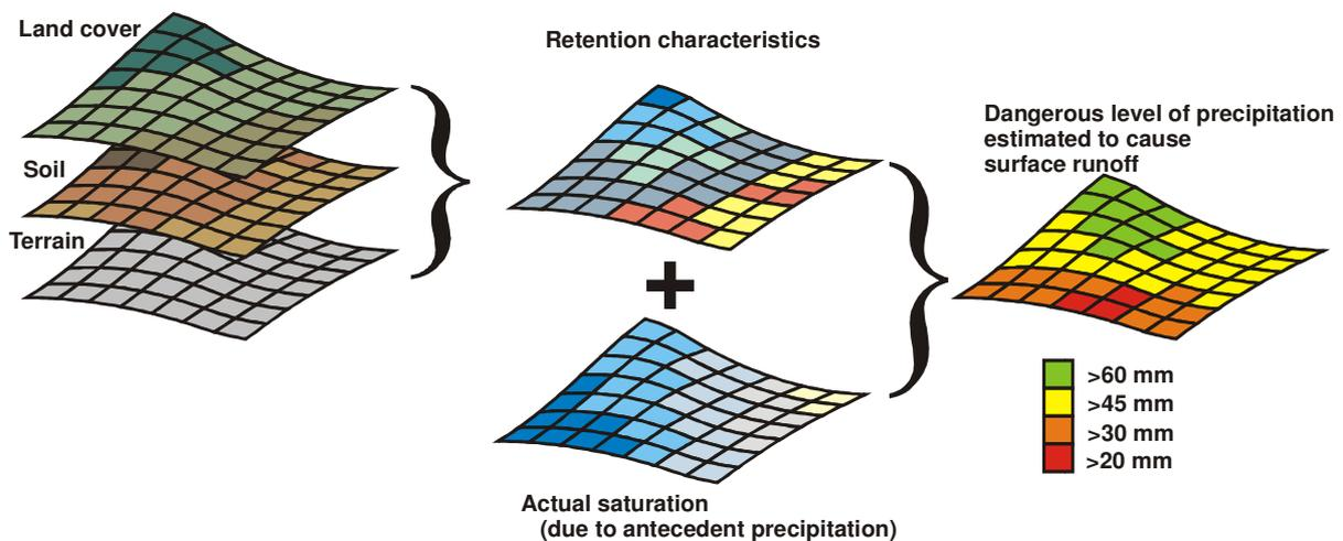
**Figure 5.** Flash flood guidance general principle – retention characteristics are described by CN value, while actual saturation is accounted through CN value update based on precipitation in last 30 days.
