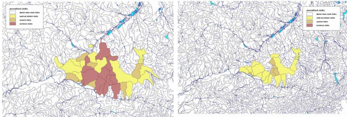
**Figure 6.** FFG-CZ a simulation of a June 24<sup>th</sup> 2009 flash flood in Nový Jičín district. Hindcast of flash flood risk level for adjusted radar rainfall estimate (left) and raw radar rainfall estimate (right) for 15:30 19:30 UTC.
