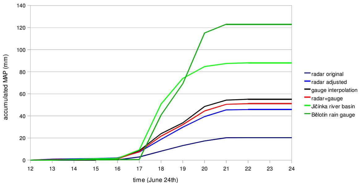
**Figure 2.** Comparison of radar estimates and rain gauge measurements over the Nový Jičín district during June 2009 24<sup>th</sup>. The evaluated amount of rainfall reached 124 mm in about 3 hours in Bělotín rain gauge.
