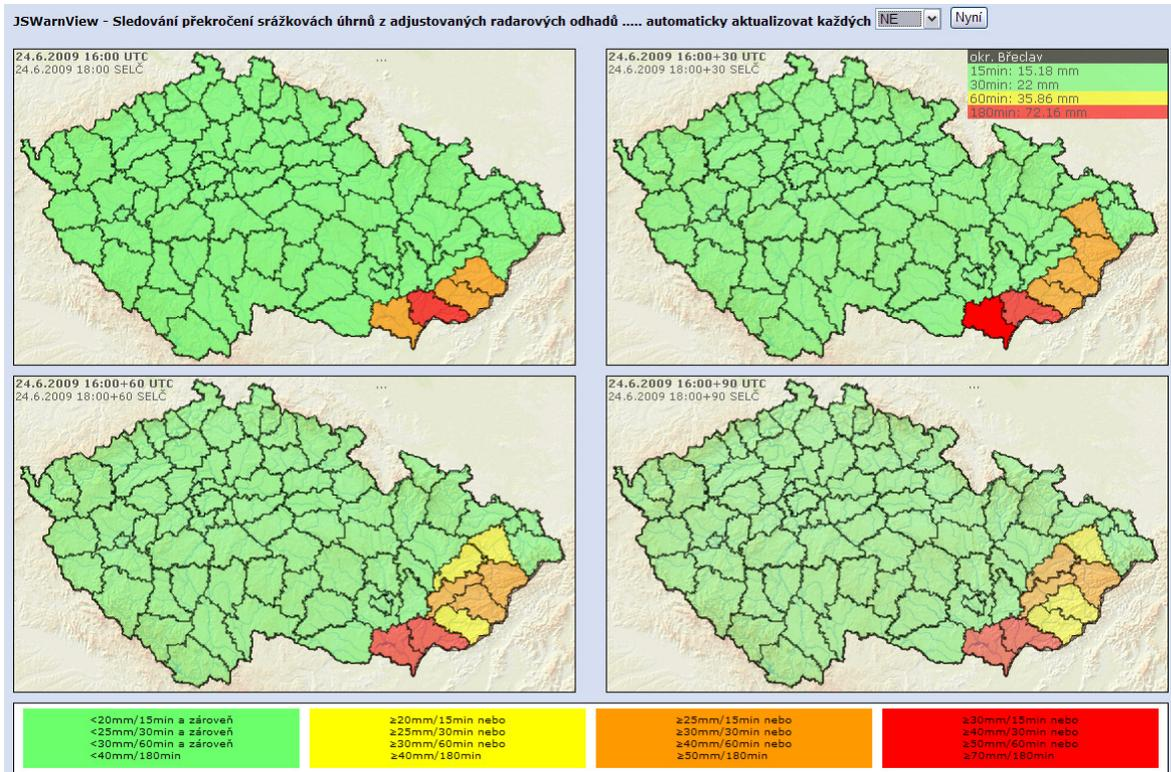
**Figure 3.** Warnview – a tool for real time evaluation of maximum radar estimates at district level for observation and three nowcasting horizons – case of June 24<sup>th</sup> 2009.
