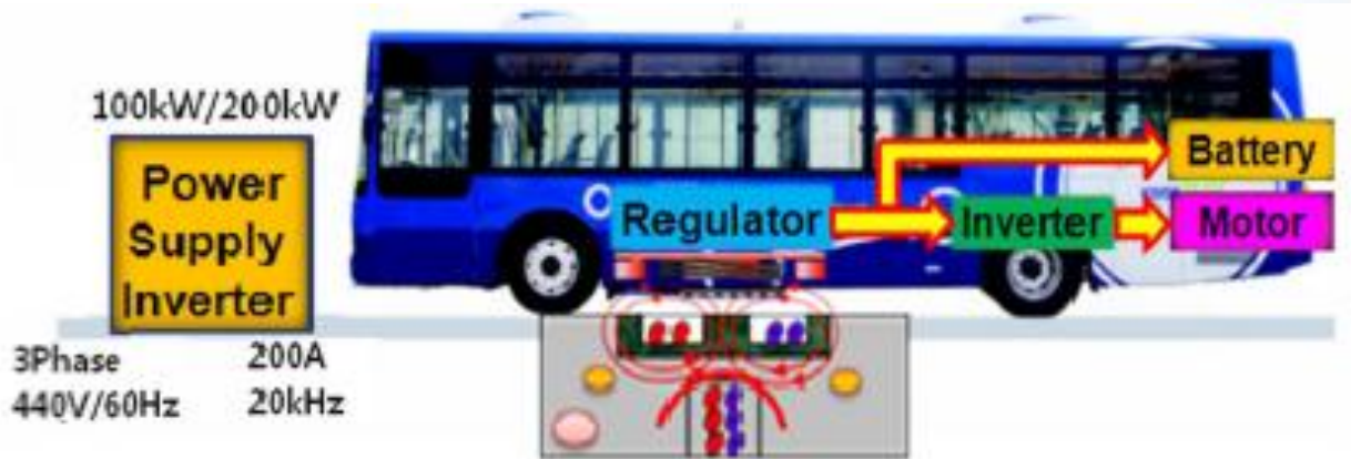
Figure 5: Schematic diagram of SMFIR technology system [9]
