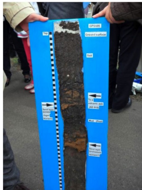
Fig. 1 – Above: the devastating tsunami occurred on March 11, 2011 along the Eastern coast of Japan. Below: tsunami deposits in the Sendai coastal plain related to the AD 869 Jogan tsunami event (Okumura, 2011).
