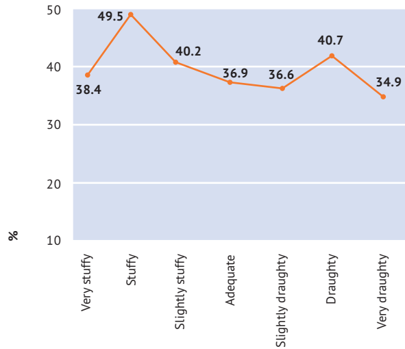
FIGURE 24: Measured mean relative humidity (%) and perceptions of ventilation in the classroom
