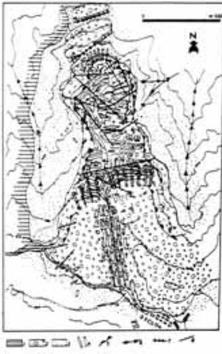
Figure 2.5 - Schematic geomorphological map of the Bisaccia area. Legend: 1. “varicoloured clays”; 2. conglomerates; 3. debris; 4. main landslide escarpment; 5. edge of the conglomerate platform scarp retreating by mass movements; 6. stream erosion; 7. trench; 8. minor landslide scarps and fractures reactivated by the November 1980 earthquake (after Crescenti et al., 1984, modified).
