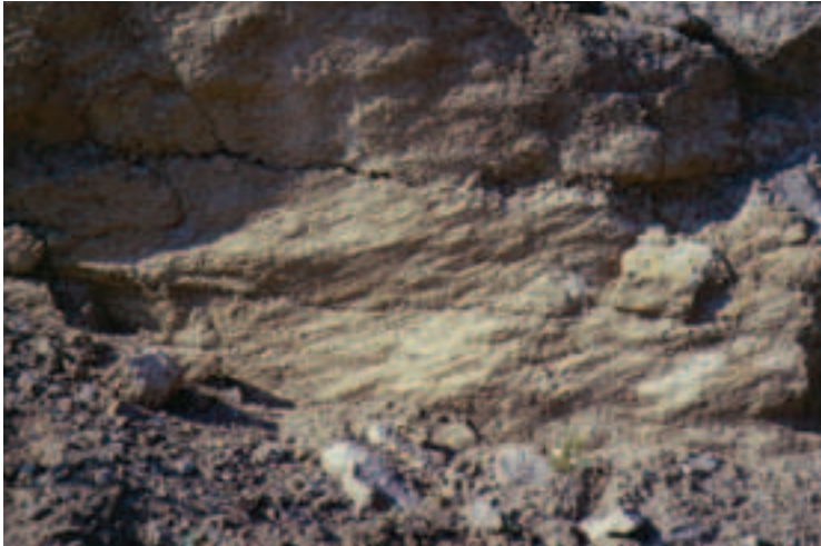
Photo 6.7 - Fault surface with striations of the Pramoritza fault zone. View from the North.
