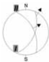
Figure 45 - Lower hemisphere projection of the average fault surfaces occurring at Mavropigi village of the Mavrodendri - Pontokomi - Mavropigi fault zone.
