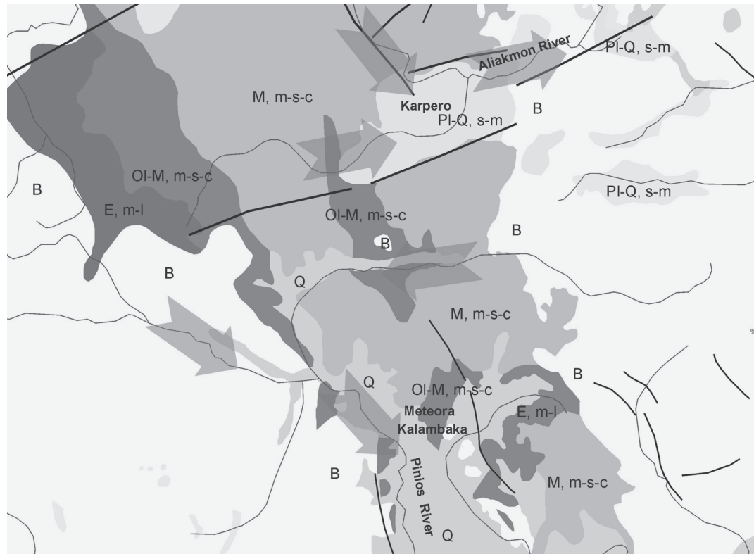
Figure 50 - Schematic geological map showing the area of the drainage divide between the Aliakmon and Pinios drainage basins. B: Alpine basement, E,m-l: Upper Eocene marls and limestones, Ol-M, m-s-c: Oligocene - Miocene marls, sandstones, conglomerates, M, m-s-c: Miocene marls, sandstones, conglomerates, Pl-Q, s-m: Pliocene-Quaternary sands, marls, Q: Quaternary deposits
