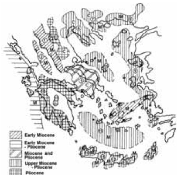
Figure 9 - Main Neogene basins of the Aegean region (after Dermitzakis and Papanikolaou, 1981): a) Lower Miocene, b) Lower Miocene – Pliocene, c) Miocene and Pliocene, d) Upper Miocene – Pliocene, e) Pliocene (M: marine, C: continental). 1: Meso-Hellenic Trough, 2: Epirus, 3: Cyclades, 4: Ionian islands, 5: Attica – Boeotia, 6: Thessaloniki, 7: Strymon, 8: Thrace, 9: Eastern Aegean islands, 10: Chania, 11: Rethymno, 12: Irakleio, 13: Ierapetra, 14: Karpathos, 15: Cretan basin, 16: N. Sporades, 17: Servia – Ptolemais, 18: Peloponnesus).
