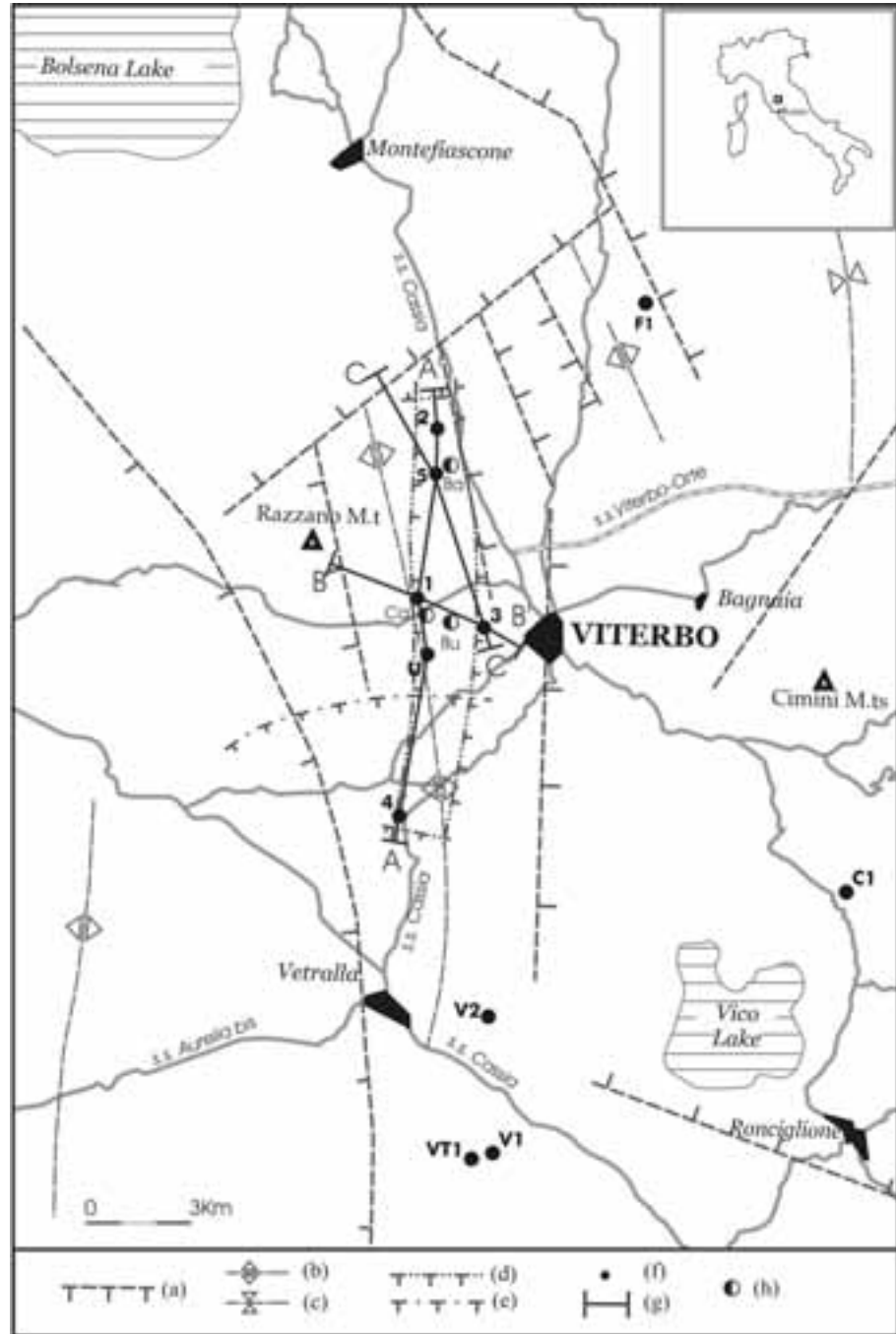
Figure 1 - Location of the Viterbo area and its main structural features. a) normal fault; b) main positive structural axis and c) main negative structural axis, obtained by gravimetric survey; d) normal fault obtained by seismic and geoelectric survey; e) normal fault detected on the base of field evidence; f) drilling by the Terny Company (1, 2, 3, 4, 5), INPS (U) and wells of ENEL and ENEL-AGIP joint venture (F1, C1, V1, V2, VT1); g) location of the stratigraphic - structural sections A - A', B - B', C - C' (cfr. fig. 4); h) main thermomineral springs (Ba, Bagnaccio; Ca, S. Caterina; Bu, Bullicame).
