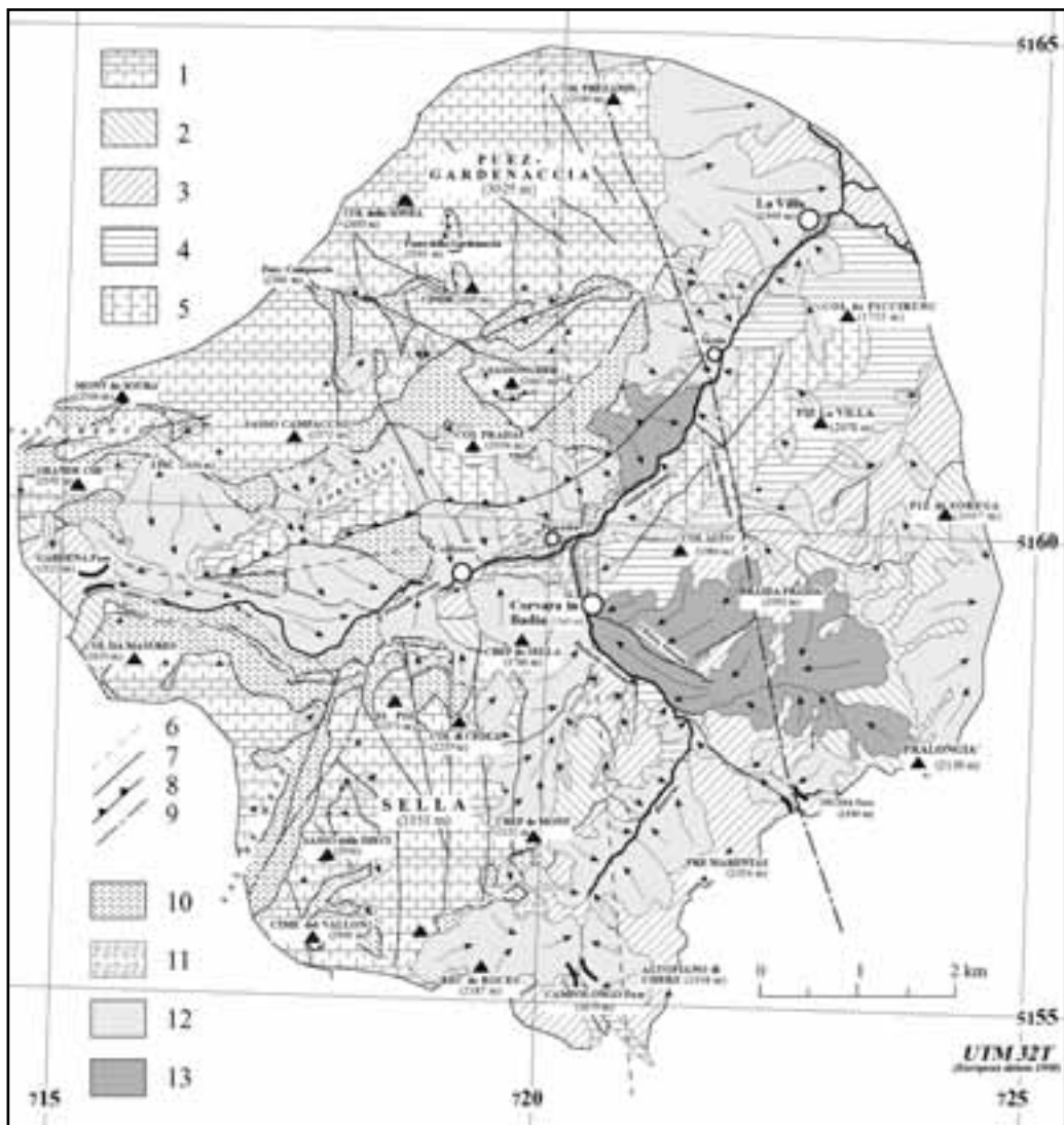
Figure 17 - Geological schematic map of the Corvara in Badia area. Legend: 1) dolomites and marls (Middle and Upper Triassic); 2) alternances of calcarenites, marls and claystones (Middle and Upper Triassic); 3) alternances of sandstones and siltstones (Middle Triassic); 4) volcanoclastic arenites and conglomerates (Middle Triassic); 5) limestones, sandstones and marls (Upper Permian-Lower Triassic); 6) palaeotectonic line (Upper Permian-Lower Triassic); 7) meso-neoalpine fault (Tertiary); 8) meso-neoalpine overthrust (Tertiary); 9) neotectonic fault (Plio-Quaternary); 10) scree slopes, scree fans (Lateglacial-Holocene); 11) alluvial or lacustrine deposit (Lateglacial-Holocene); 12) landslide (Lateglacial-Holocene); 13) Corvara and Col Maladat landslides (after Corsini et al., 2001).
