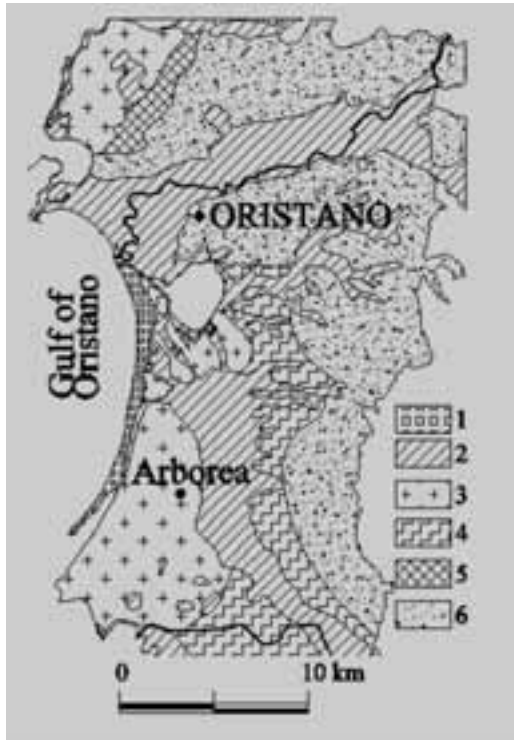
Figure 29 - Geological map of the Oristano plain. Holocene: 1. Present and recent beach sands passing to coastal dunes; 2. Pebbly-sandy or clayey alluvia and clayey silt palustrine or brackish deposits. Pleistocene: 3. More or less cemented dune sands; 4. Pebbly-sandy alluvia covered primarily with (ancient) relict dunes; 5. Pebbly terraced alluvial deposits with interbedded sand; 6. Pebbly alluvial deposits of the upper terraces.
