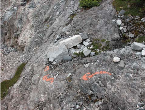
Fig. 16 – Black benchmark (red in the field), now in disuse, used for measuring the frontal variations of the glacier tongue. Numbers and acronyms codify the mark and refer to the glaciological operator and to the year in which the bench mark was placed (photo by Carton, 2004).
