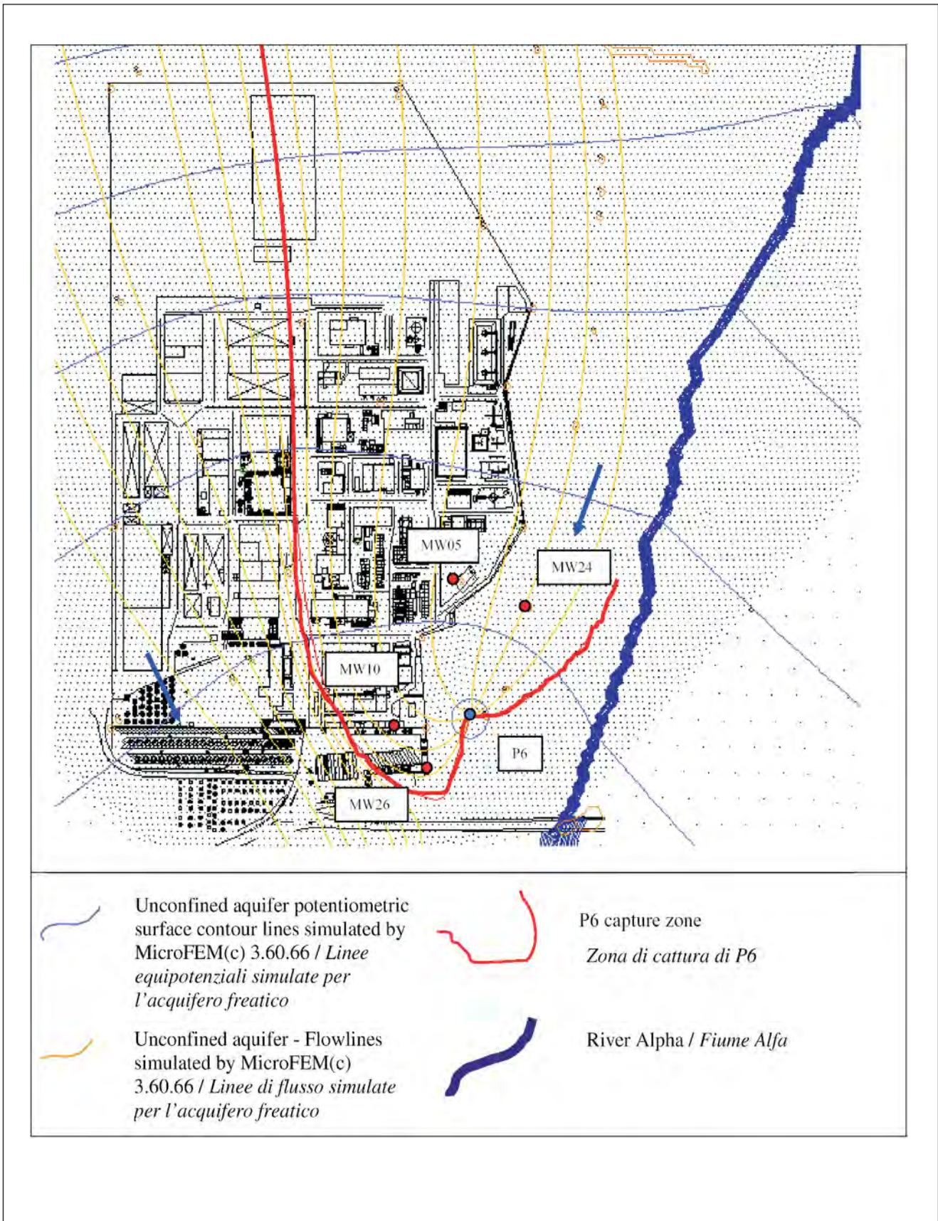
Fig. 10 - Simulated flowlines in the upper unconfined aquifer with well P6 pumping at 140 m<sup>3</sup>/hour.
