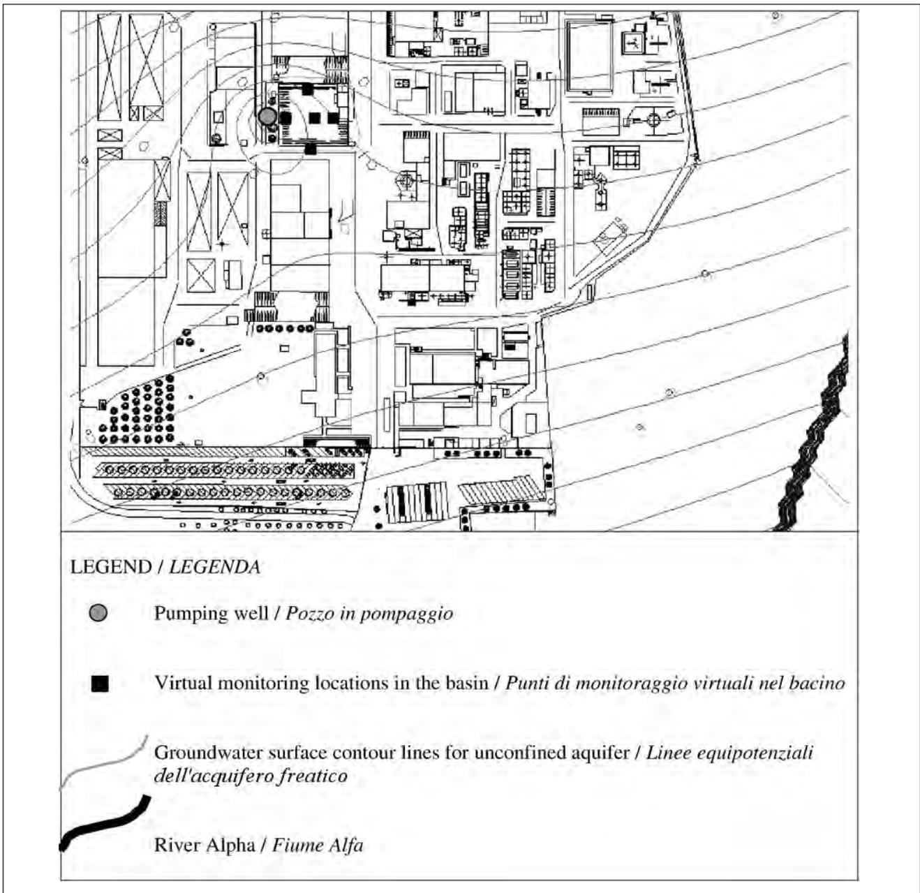
Fig. 12 - Location of pumping well and virtual monitoring locations selected to simulate drawdown inside the basin.
