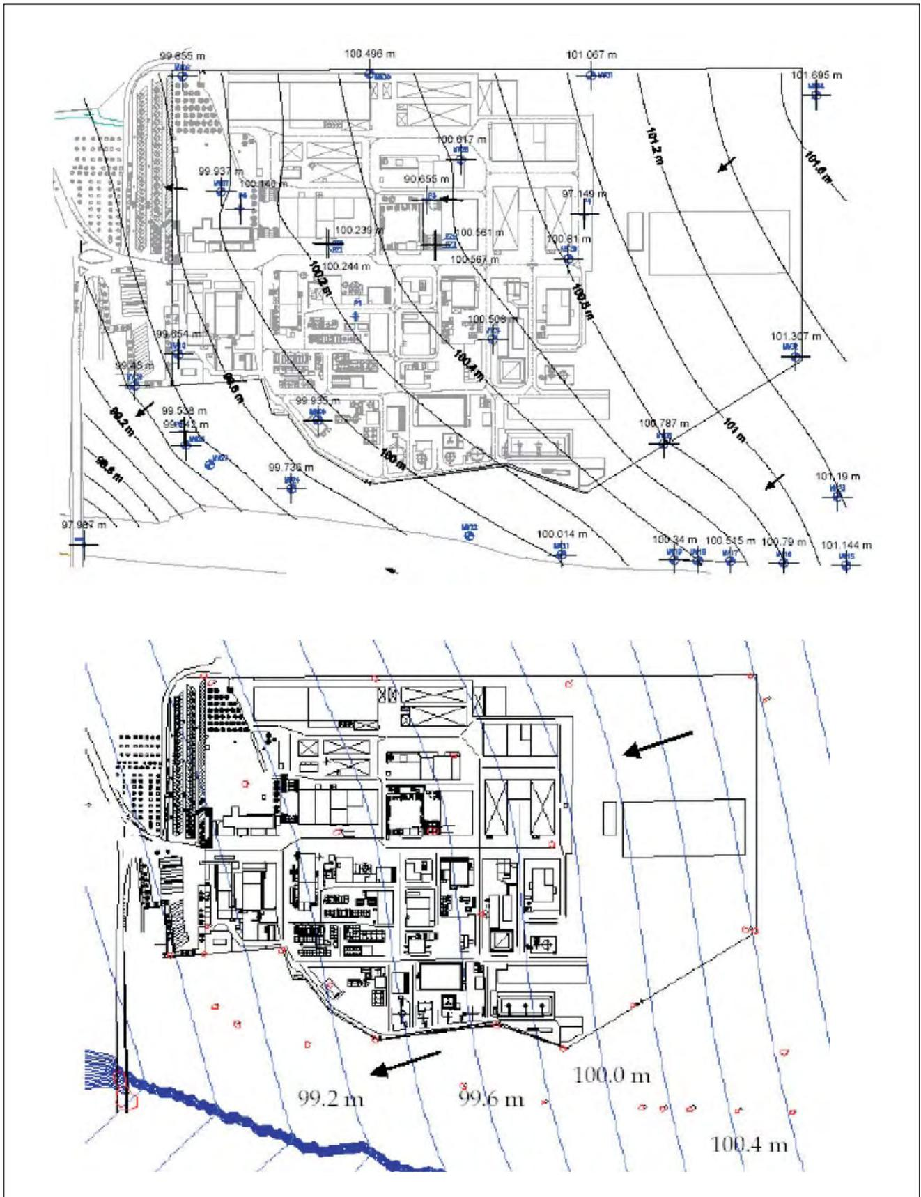
Fig. 8 - Comparison between measured data (above) and simulated data (below) – Groundwater surface map for the unconfined aquifer.
