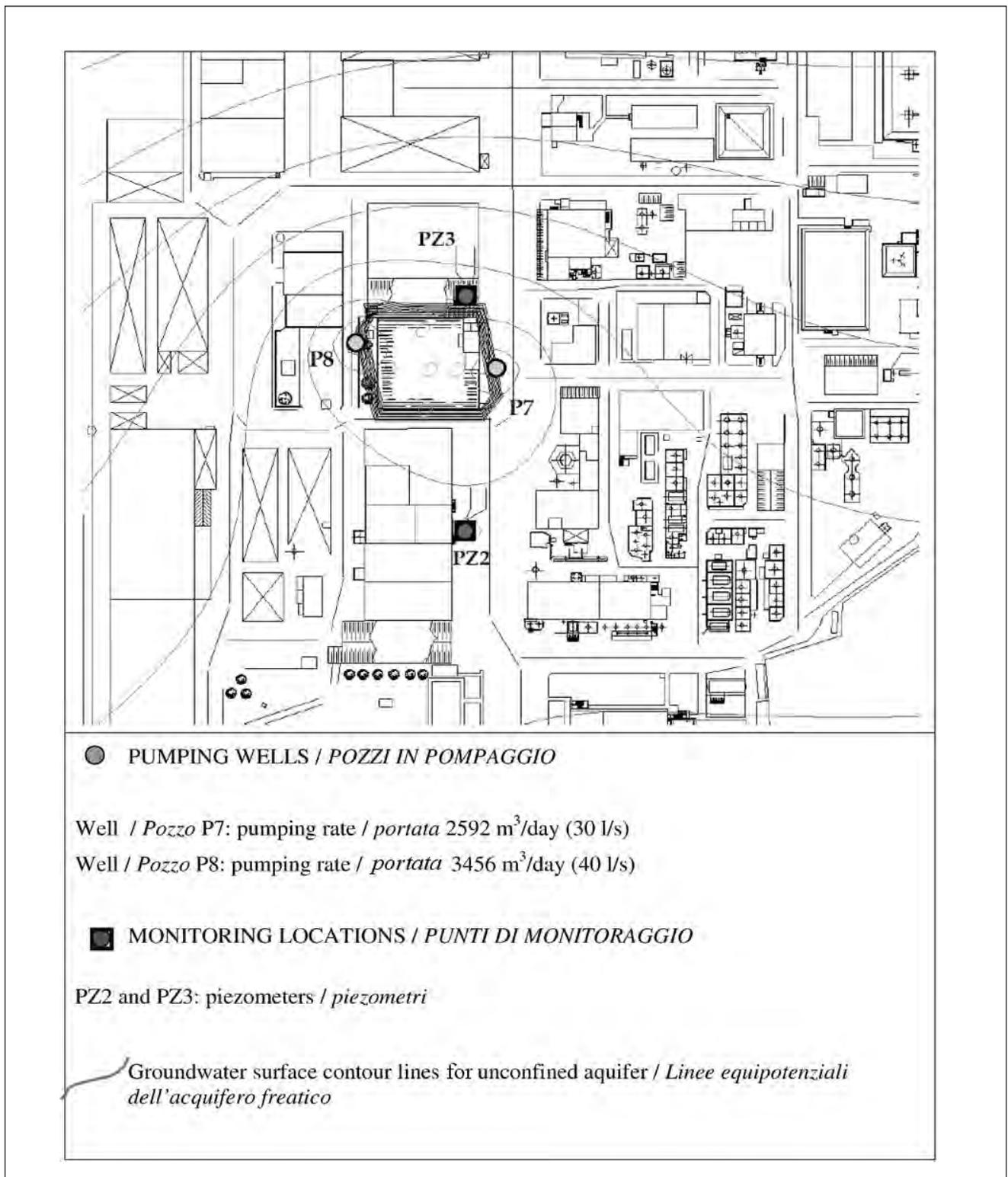
Fig. 13 - Groundwater surface map simulated for the unconfined aquifer at the end of the 26 hours-pumping test.
