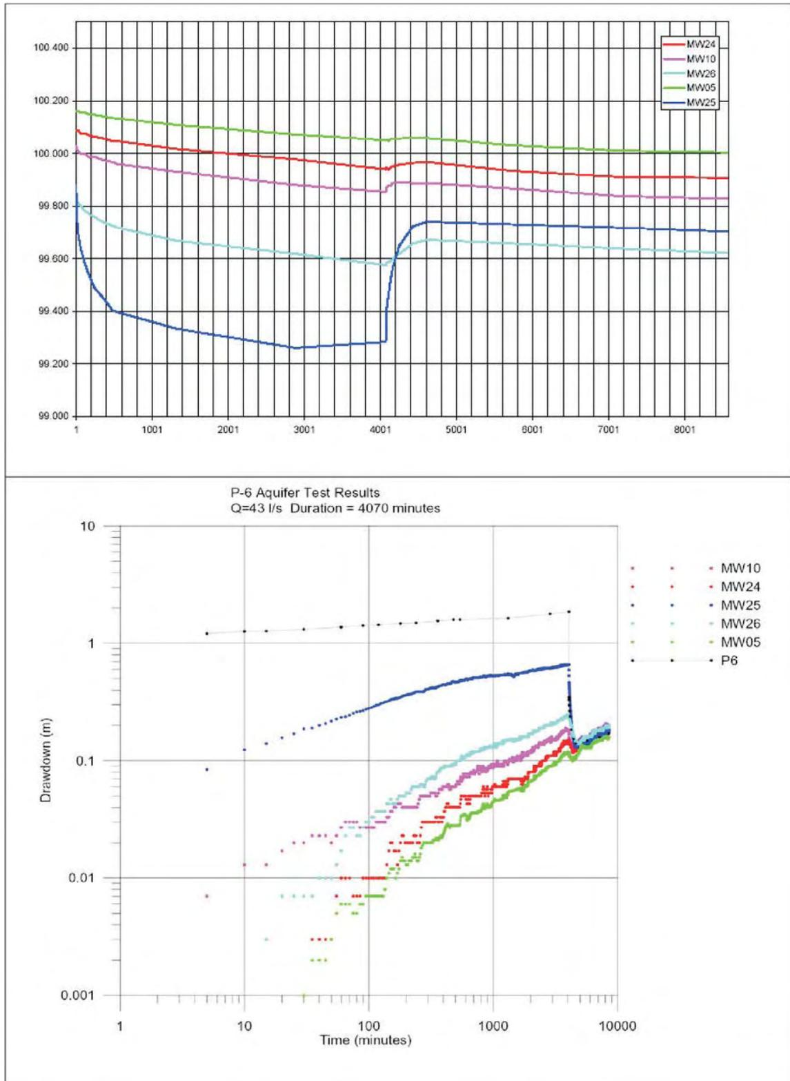
Fig. 7 - Comparison between measured drawdown (above) and simulated drawdown (below) – PRT interpretation using the MLU software.
