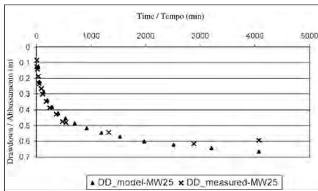
Fig. 6 - Comparison between simulated and measured drawdown during constant discharge (Pump and Recovery Test - PRT) at P6.
