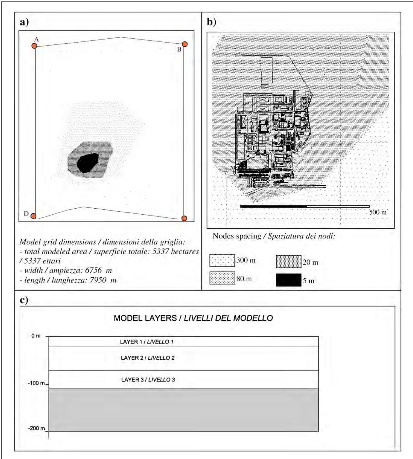
Fig. 3 - Groundwater flow model configuration. a) Model grid dimensions, b) Model grid: detail of the chemical facility area, c) Model layers.
