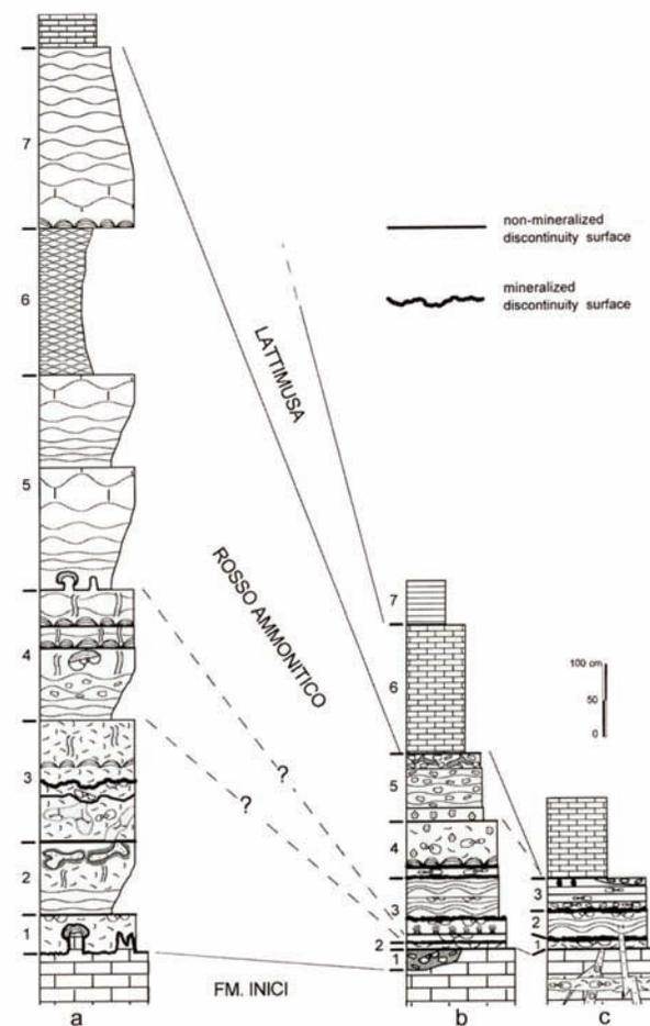
Stratigraphic logs of the measured section. *a)* Poggio Roccione, *b)* Rocca chi Parra central part, *c)* Rocca chi Parra western side. Correlation lines are traced mainly on the basis of lithostratigraphical criteria. Hatched lines with question marks indicate only hypothetical correlations.
