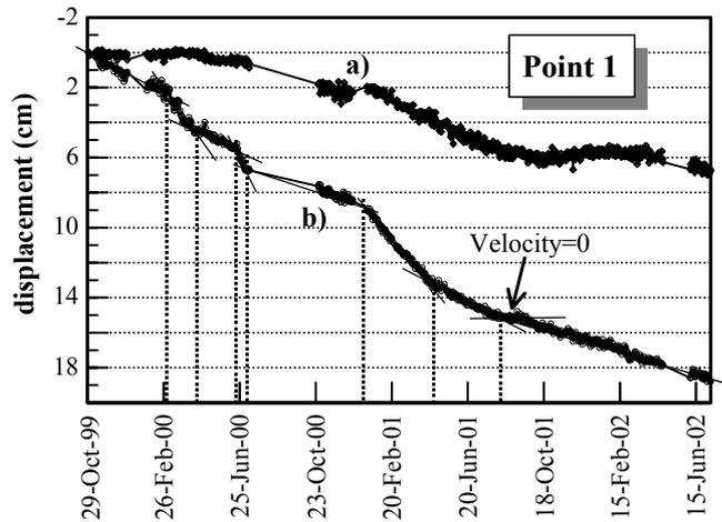
Fig. 7. Trend of the altimetric (a) and planimetric (b) components of the movements measured at point 1, and details of the periods in which the speed remains constant.
