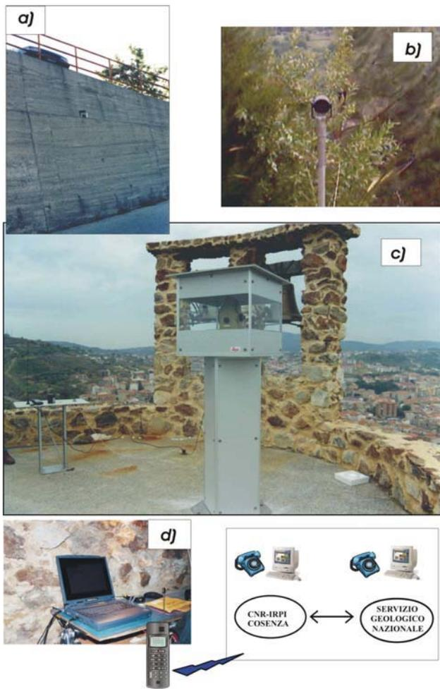
Fig. 4. Elements of the surface movement monitoring network: a) reference point, b) measurement point, c) total station, d) computer.
