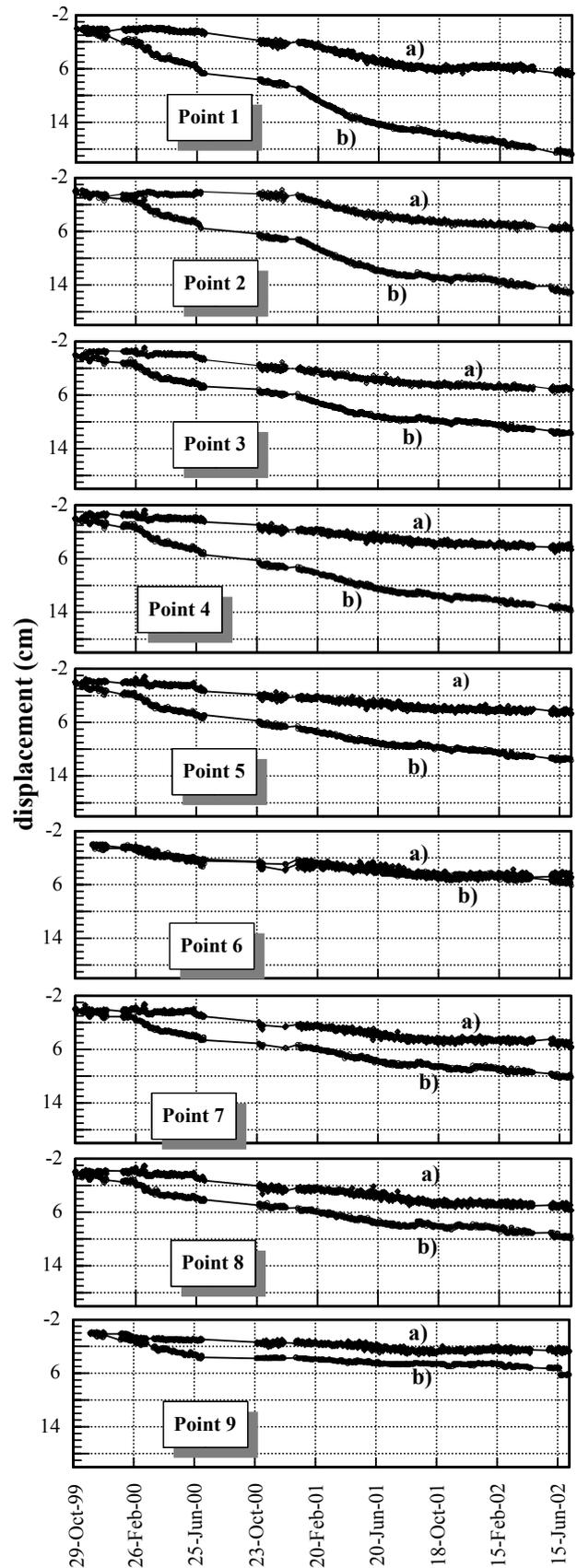
Fig. 5. Trend of the altimetric (a) and planimetric (b) components of the movements surveyed at the measurement points.
