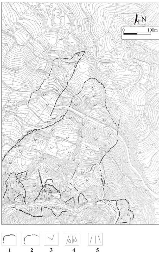
Fig. 2. Limit of area concerned with 1998-1999 remobilization. Legend: 1= landslide crown; 2 = landslide limit; 3 = type of movement (sliding); 4 = debris deposits with large blocks; 5 = debris deposits. From Sorriso-Valvo *et al.* (2001).
