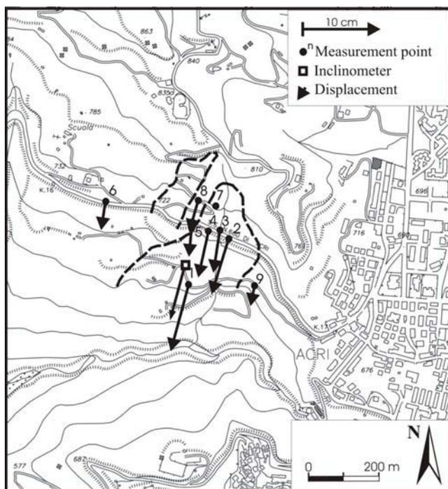
Fig. 6. Movements accrued between 12/1/01 and 8/7/02 and measurement of the movement at 1 m above ground level along the vertical line of inclinometer S3 during the same period of time.
