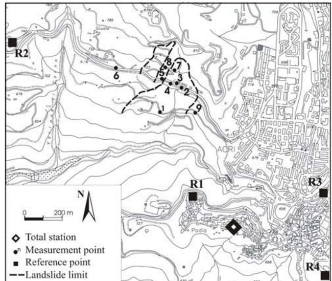
Fig. 3. Configuration of network for monitoring surface movements.
