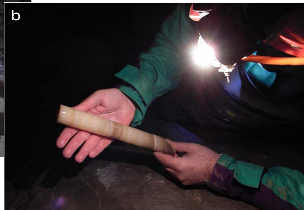
Fig. 3.11 - a) Drilling operation within the "Laghetto basso"; b) The CD3 just extracted: it contains ca. 1 Ma of climate history.
