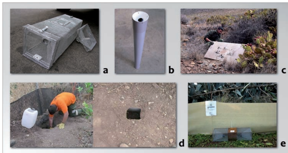
Fig. 6. Kinds of traps tested (a. funnel trap; b. PVC funnel trap; c. artificial covers; d. pitfall trap; e. artificial barriers with funnel trap). The artificial covers consist of 60 x 120 x 14 cm wooden boards. Photos a, b, d y e: José Miguel Sánchez Rivero. Photo c: Alejandro Ramírez Reyes.
