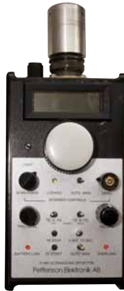
Figure 4.18 - Pettersson D980 bat detector. This device allows ultrasound to be converted into audible signals. Three different functions are allowed: heterodyne, frequency division and time expansion.
